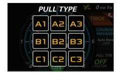
speed. The lower the letter (A being the lowest) the longer it will take for the engine to respond to the speed drop. The higher the letter (C being the highest) the faster the engine will respond to the speed drop.
