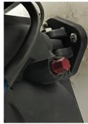
For the Power Wedge III, using a small (stubby) straight screwdriver, loosen the small red screw on the actuator beneath the swim board until it stops. Lift or lower the wedge to the position desired and then tighten the screw snugly (but do not over-tighten). Manually cycle the wedge a couple of times after doing this to ensure that the screw is snug, and the wedge moves correctly.
