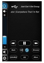
Touch *USB* to access a device plugged into the dash USB port. *USB Input Devices* with music stored on them are accessed from this screen.
