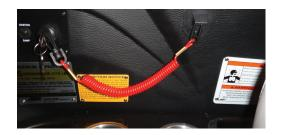
The switch assembly consists of an ON-OFF switch and a switch/lanyard clip. The engine will not start and/or run if the toggle is in the OFF position. Malibu recommends the clip always be inserted in the toggle switch. Connected to the operator, if (s)he moves away from the controls, the clip will pull free, pulling the switch to the OFF position. If the engine needs to be shut down very quickly, it can be done so by pulling on the lanyard to release it from the switch.
