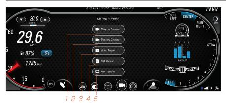
With the Backup Camera option and/or Docking Camera option turned ON in the Settings menu, the buttons for the camera feeds will be selectable.
