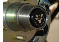
The system has several unique features not found on conventional trailer axles. Every possible leak point on the front and rear of the hub is sealed. (The slight pressure inside the hub is needed to keep water out of the hub chamber when the hub is submerged underwater during loading and unloading).
