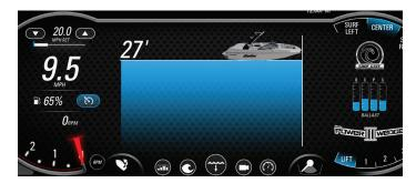
Touch the *Depth* button at the bottom of the 12" display screen to view the current water depth. This page will also show the driver the last twenty (20) seconds of Depth history.
