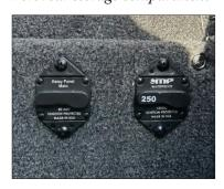
There are two breakers located on the board in the port rear closeout, adjacent to the engine compartment. The breaker labeled Relay Panel Main controls the Power Wedge III and Surf Gates. The one stamped with 250 controls the Stern Turn (if equipped). If any of these systems will not operate, verify that the supplemental breakers located in the port rear storage compartment are properly set.
