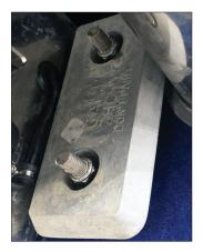
Important Note: The sacrificial zinc anode does not eliminate the corrosion process. Therefore, it is important to flush and rinse the boat after use.
