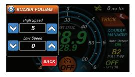
appears: Select the volume for High and Low speed by utilizing the up and own arrows. Touch *Back* to return to the *Slalom Settings* screen.
