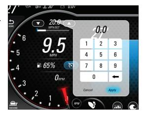
**Step 7:** Select the desired Wedge Position. This can be set to Lift through Stow. Press the *Next* button when the Wedge position is set.
