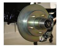
Because the wheels and hubs will be submerged in water at times, they require more attention than those found on a tow vehicle. Wheels should be regularly washed with mild soap or detergent to retain the finish and remove any corrosive elements. Never use harsh detergent or scrub brushes that can damage the appearance.
