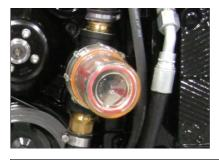
Most often, the cause of overheating is either marine growth clogging the raw water intake or insufficient coolant/water. If there is debris, even in small amounts, in the body of water, during usage it is likely that some of the marine growth can accumulate in the cooling system.
