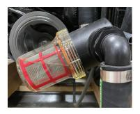
The raw water intake/sea strainer must always be free of debris. Any boating that takes place in brackish water or water with flora, should be interrupted periodically to be certain that no weeds have become tangled with anything under the hull. See the *Care and Maintenance* section in this manual for information on how to properly remove debris from the raw water intake/sea strainer.
