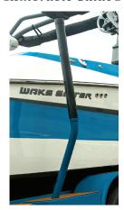
Malibu trailers are equipped with removable guide poles as standard equipment. The poles, located on each side of the trailer, assist in assessing the total width of the boat and trailer relative to towing or while backing up, as well as parking the trailer and boat inside/under shelter such as a garage.
