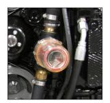
As part of the routine annual maintenance, the raw water pump should be inspected, with particular attention to the impeller. The process for inspection is explained in the *Care and Maintenance* section of this manual. **If the boat is operated in shallow or brackish**
