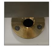
All boats are equipped with two drain plugs, a 1/2" drain plug on the transom and a T-handle drain plug in the center of the boat. The 1/2" drain plug can be accessed outside the boat, directly under the swim platform on the center back of the transom. The T-handle can be accessed inside the boat through the center access. Be certain to read the above information regarding **SECURELY** installing drain plugs prior to all outings.
