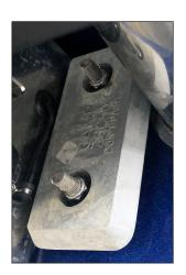
One of the most important saltwater components is the sacrificial zinc anodes. These are attached to the exterior of the boat, below the water line.
