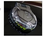
Therefore, care should always be taken while fueling the boat. Do not stand too close to the fuel fill location in case some fuel is expelled from the pressurized system. You may also hear an audible release of air pressure when opening the cap. Pay attention to ensure that gasoline is entering only into the boat's fuel fill and not spilling or running outside the fuel fill.
