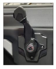
When engaging the transmission from Neutral either forward or backward into reverse, pull up on the safety collar located directly below the throttle lever knob. The safety collar helps avoid unintentional movement into gear.
