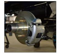
The trailer brakes should always be maintained in top condition. This includes regularly checking the fluid level in the actuator. The loss of brake function can result in loss of control or the inability to stop the trailer, which could lead to serious injury or death.
