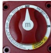
both battery banks ON or OFF or to combine. The advantage to this system is that it allows the operator to direct power draw from each bank individually or combine both banks to take advantage of a larger battery system when needed.
