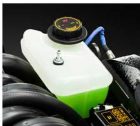
percent extended warranty antifreeze plus 50 percent distilled water. (Do not use tap or other water as other elements in the water can cause build ups or deposits within the closed cooling system. This can interfere with proper operation and resulting damage is not covered under warranty.)
