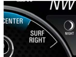
The NIGHT mode button toggles the backlighting between the DAYTIME and NIGHTTIME set points that can be found in the SETTINGS menu. NIGHT MODE not only controls the brightness of the screens, it also controls the lighting of the various buttons found on the dash and the optional Sport Dash rotary controller.
