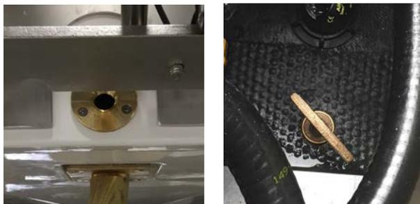
All boats are equipped with two drain plugs, a ½" drain plug on the transom and a T-handle drain plug in the center of the boat. The ½" drain plug can be accessed outside the boat, directly under the swim platform on the enter back of the transom. The T-handle can be accessed inside the boat through the center access. Be certain to read the above information regarding securely installing drain plugs prior to all outings.
