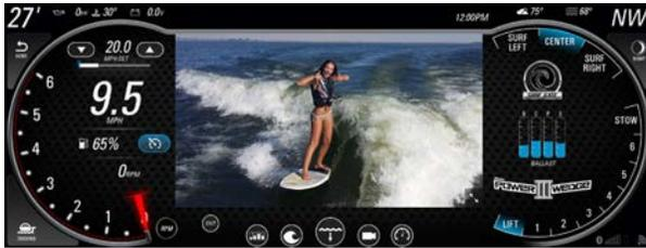
With the Reverse Camera option turned ON in the settings menu, the button for the camera feed will be selectable. This camera feed will bring up the camera that is mounted to the transom of the vessel.
