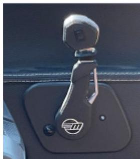
To the right of the boat operator is the shift/throttle lever. Any time the boat engine is off, the lever should be in the center upright position, which is Neutral (meaning the boat is not in gear) and is apparent when it can be felt slotting in with an auditory click. Boats are not equipped with “Park” like land-based vehicles.
