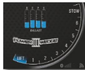
The Power Wedge is not intended for use at speeds greater than 26 mph. A notice will be displayed if the Power Wedge is in a deployed position at speeds exceeding 26 mph. Boat speed must be below 26 mph to dismiss the alarm. The Power Wedge
