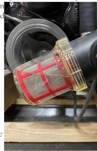
*and Maintenance* section in this manual for information on how to properly remove debris from the raw-water intake/sea strainer.
