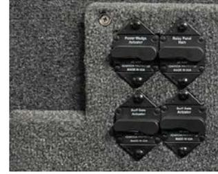
Power Wedge III, Surf Gate, and Stern Turn (if equipped) breakers are located on the board in the port rear closeout adjacent to the engine compartment. If any of these systems will not operate, verify that the supplemental breakers located in the port rear storage compartment are properly set.
