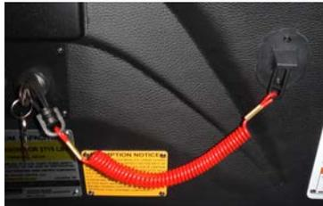
Your boat is equipped with an Emergency Safety Lanyard (cutoff switch). We recommend that the lanyard be secured to the operator and
