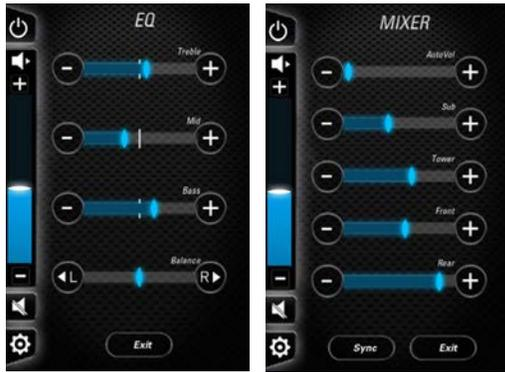
The Equalizer page allows the driver to adjust the treble, mid, bass, and balance. It is recommended to leave the treble, mid, and bass centered at zero.
