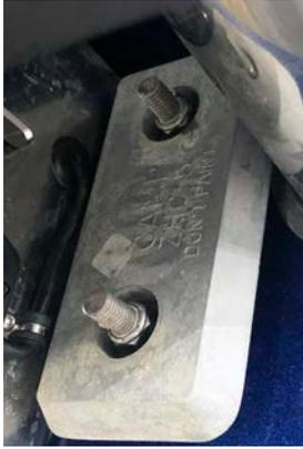
(oxidation) and metal reduction are the effects of operating in saltwater. To reduce these naturally occurring results on boat components, the sacrificial anodes attract and reduce most of the effects.
