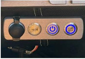
On a boat equipped with a Start-Stop button, press the button. If you are using the backup key, also turn the key to OFF. (Failing to do so means the electrical system will continue to function;
