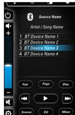
of paired devices. If the desired device has been paired and is within range, the user can connect to the device from the 7" screen.
