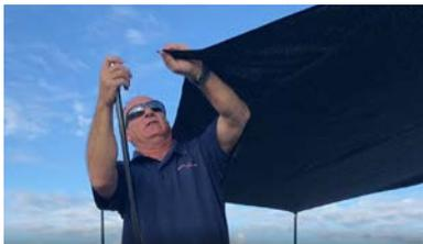
5. On the front, attach the canvas around the aft hoop(s) in the corners on the G5 or GX.
