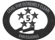
**Five Star – Level Five Extremely Clean.** The five star label identifies engines that meet the Air Resources Board's Voluntary Standards for spark-ignition marine engines. Engines meeting these standards have 50% lower emissions than Four Star–Super Ultra Low Emission engines.
