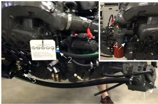
*The engine drain plugs are located: 1. The V-drive 2. The bank 1 manifold, 3. Under the heat exchanger and 4. The bank 2 manifold.*
