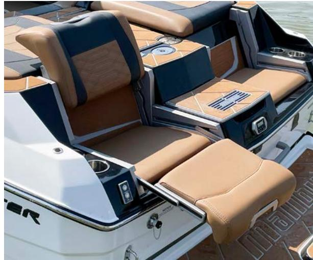
No one should sit or ride on the sun pads when the boat engine is running. Carbon monoxide is emitted from the exhaust system and vented into the water beneath the swim board. Fumes can and do reach the sun pad area. Avoidance of carbon monoxide poisoning is addressed in the *Safety* section of this manual.
