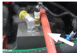
pinched. If it is possible to alleviate this situation safely, then do so. The preferable method, however, is to have an authorized Malibu dealer's trained service technician do so and verify that no damage has been done to the line or other equipment.
