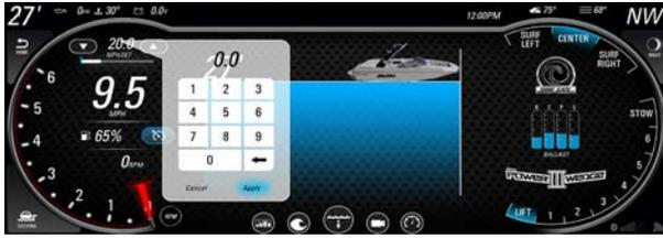
1. With the engine running and in neutral, turn the speed control on by touching Speed Control button. The button will turn blue, and the speed control information will appear above the boat's speed reading.
