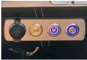
On a boat equipped with a Start-Stop button, press the button. If you are using the backup key, also turn the key to OFF. (Failing to do so means the electrical system will continue to function;
