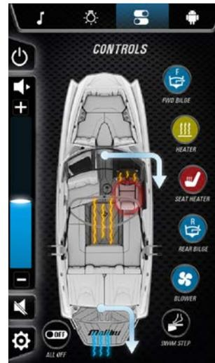
Touch the Forward Bilge to turn the forward bilge pump ON and OFF. If an Auto-Bilge Alert occurs, the driver will be able to navigate to the Controls page to see which bilge pump is running.
