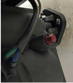
the wedge moves correctly. For the Surf Gate, there is a red hex bolt on the side of the actuator. Opening this valve with a 3/8" wrench will allow the Surf Gate to be moved into a closed position. Be sure to re-tighten the bolt to prevent it from drifting open while operating the boat.
