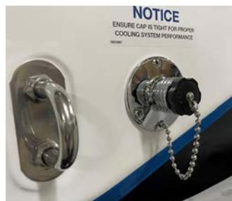
In boats equipped with the optional flush kit (which is highly recommended in boats operated in salt brackish water), the flush kit is used to clean out the raw water pickup and operational areas of the engine. The kit attachment is located on
