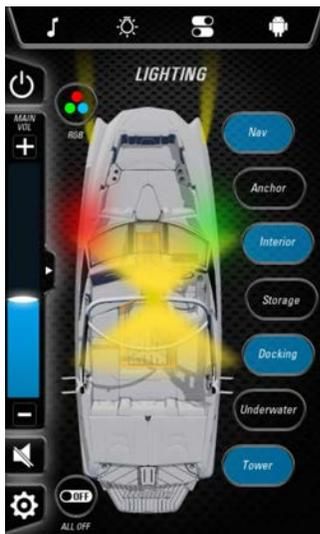
Touch Anchor to turn the Anchor Light ON/OFF.
