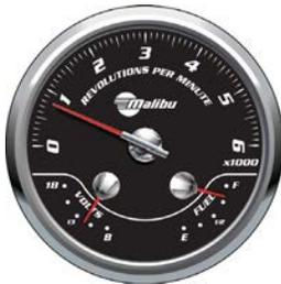
The Right Gauge is the Tachometer, which shows the engine's rotational speed in revolutions per minute. There are two smaller gauges that are built into the Tachometer. The gauge in the lower left of the Tachometer is the Battery Voltage. The desired
