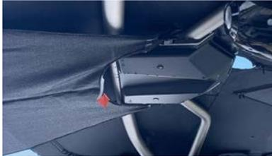
There should be enough strap length to adjust how tight the canvas is after the awning is fully deployed.
