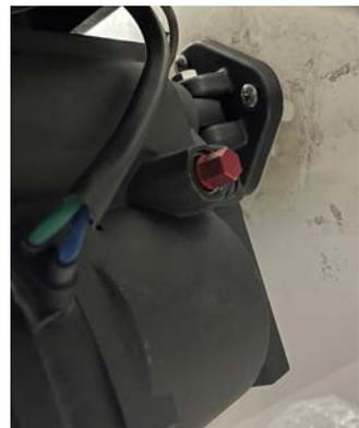
on the side of the actuator. Opening this valve with a 3/8" wrench will allow the Surf Gate to be moved into a closed position. Be sure to retighten the bolt to prevent it from drifting open while operating the boat.
