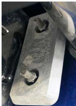
transom zinc anode via grounding wire. Anodes are also affixed to the exhaust manifolds.
