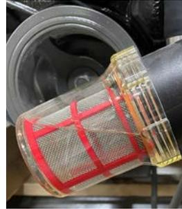
Raw water from the body of water is drawn into the boat as part of the cooling system for the engine and drive train. Even with the closed cooling systems, it is necessary to circulate additional water as part of an effective cooling system. To protect the system, a sea strainer is installed near the raw water intake, located
