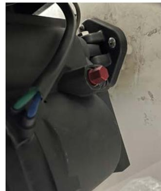
on the side of the actuator. Opening this valve with a 3/8" wrench will allow the Surf Gate to be moved into a closed position. Be sure to retighten the bolt to prevent it from drifting open while operating the boat.
