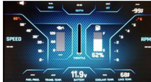
The Gauge screen will show the driver vital information that pertains to the vessel and the engine.
