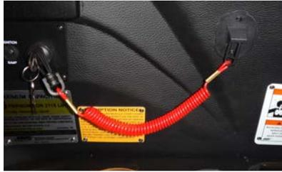
**Step 4:** Press the Power Button and check that power has been supplied to the Electrical System. The 7" Display will begin to power up.
