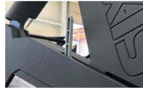
4. Flip the small gray levers up that are in the base. If they do not flip up easily try pushing the side support inboard slightly ('Axis' is machined into them).
