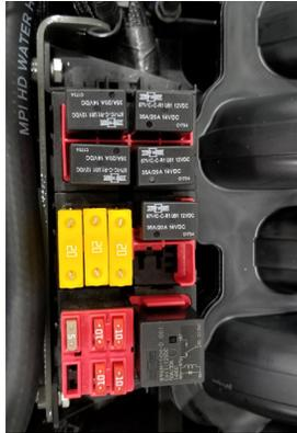
In addition to the circuit breakers that control most of the electrical activity on the boat, Axis engines also have a fuse box on the engine.
