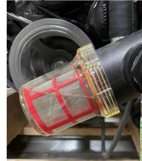
To protect the system, a sea strainer is installed near the raw water intake and serves the purpose of keeping debris from entering the cooling system, causing eventual engine failure. As with any kind of strainer, it is necessary to regularly clean it so that water can flow unimpeded.
