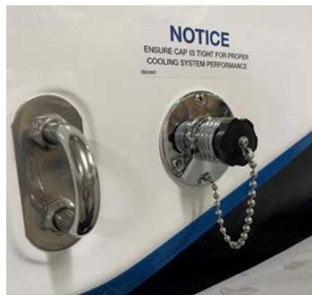
In boats equipped with the optional flush kit (which is highly recommended in boats operated in salt/brackish water), the flush kit is used to clean out the raw water pickup and operational areas of the engine. The kit attachment is located
