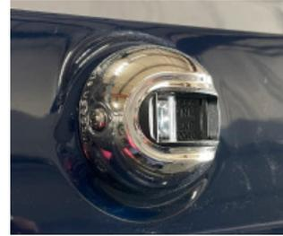
visibility. There is a green light on the starboard side and a red light on the port side, operated from a button on the dash panel. The green light will be on the starboard side of the deck adjacent to the driver's helm, and the red light will be on the port side deck adjacent to the observer seat location. The lights are controlled from a button on the dash panel.
