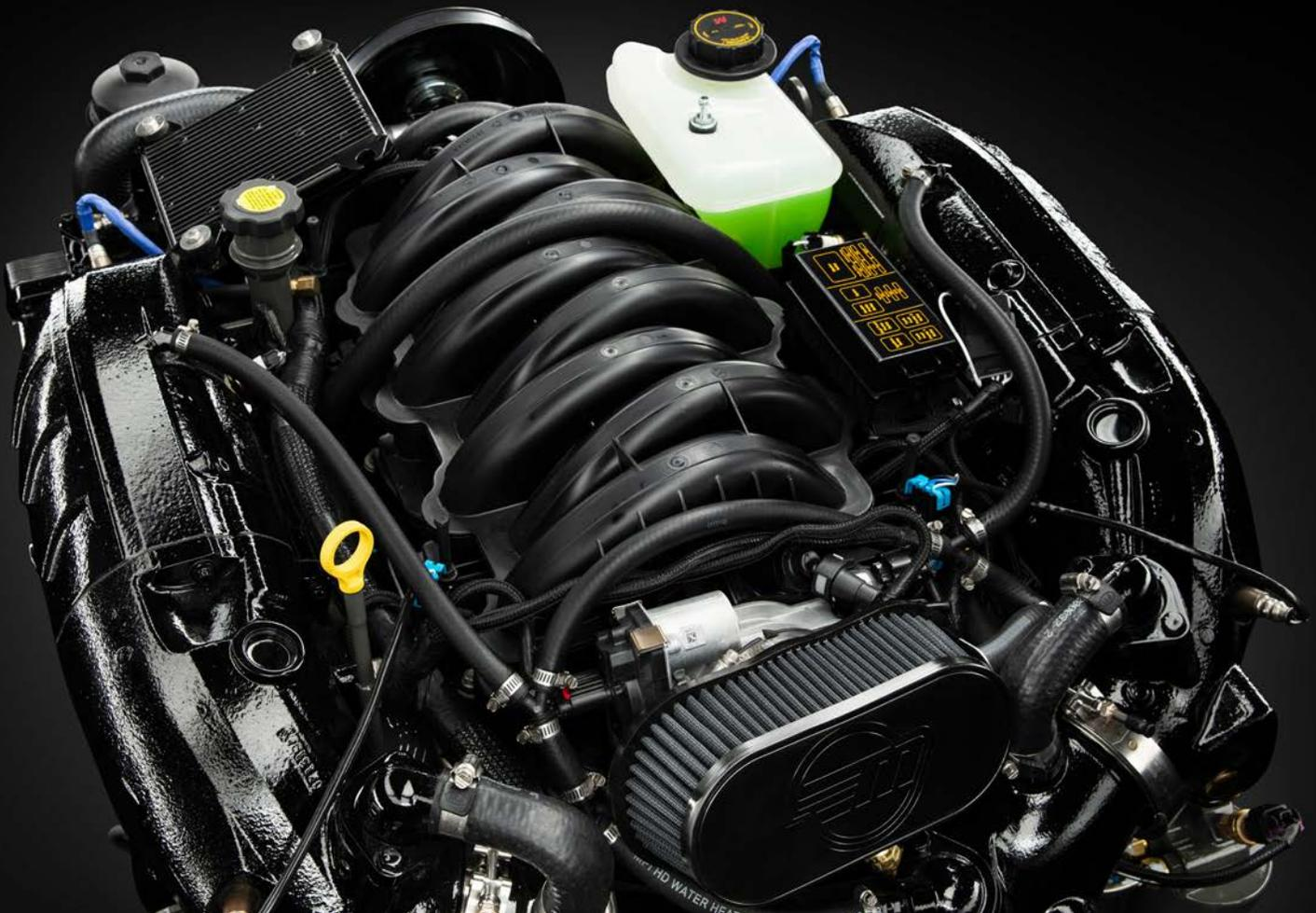
Although the Axis fuel system works very efficiently, there will always be some gaseous by-product as a result of operating an internal-combustion engine. These gases, along with the water used to cool the engine (in addition to the closed cooling system) are routed out of the boat by way of the exhaust manifolds on each side of the engine to exhaust houses between the deck and hull, and it is expelled out of the system at the transom.
