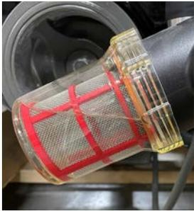
Both the paddlewheel and raw-water intake/sea strainer must **ALWAYS** be free of debris. Any boating that takes place in brackish water or water with flora, should be interrupted periodically
