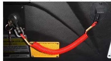
Your boat is equipped with an Emergency Safety Lanyard (cutoff switch). We recommend that the lanyard be secured to
