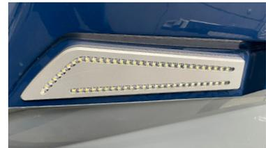
and provide white light to the front of the boat. The docking lights are operated from a screen icon.
