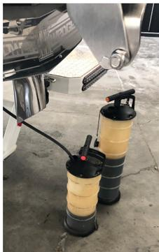
5. If a siphon pump is available, remove the drain line cap, create a seal on the siphon hose and start the pump.
