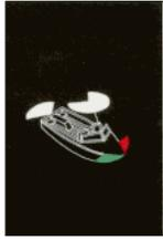
Sailboats operating under machinery, or under sail and machinery, are considered power driven and must display the lights prescribed for a power-driven boat.
