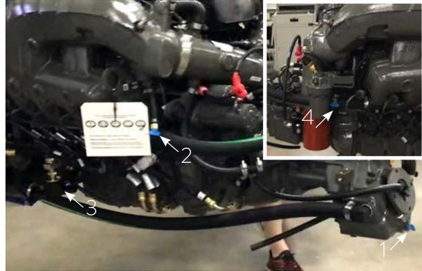
The engine drain plugs are located: 1. The V-drive 2. The bank 1 manifold. 3. Under the heat exchanger and 4. The bank 2 manifold.
