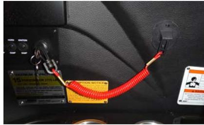
will not start and/or run if the toggle is in the OFF position. Axis recommends the clip always be inserted in the toggle switch. Connected to the operator, if (s)he moves away from the controls, the clip will pull free, pulling the switch to the OFF position. If the engine needs to be shut down very quickly, it can be done so by pulling on the lanyard to release it from the switch. To reset the switch after activation, reinstall the lanyard clip and flip the switch to the UP position.
